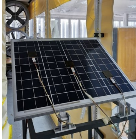
Figure 8.1. Experimental test rig layout in wind tunnel [117].
