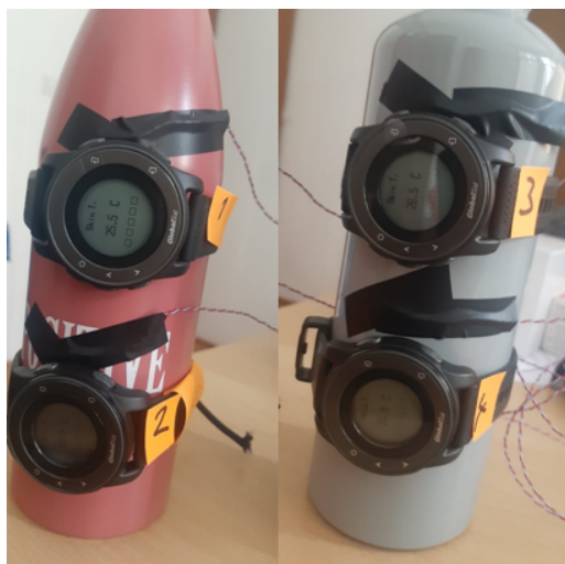
Figure 2.16. Setup for GlobalSat bracelet temperature features testing
